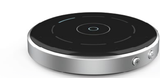
Figure 1. Table Microphone in Automatic Mode. The active direction of the beamformer is shown by the illuminated segment.
